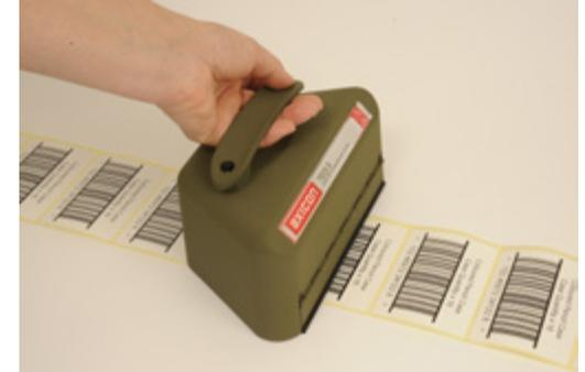
The verifier should be placed either just above or just below the barcode and the trigger pressed. With the trigger still pressed, move the verifier down the height of the barcode. The verifier will scan at the rate of 100 verifications a second until it reaches the bottom of the barcode (or gets to the maximum number of scans).
