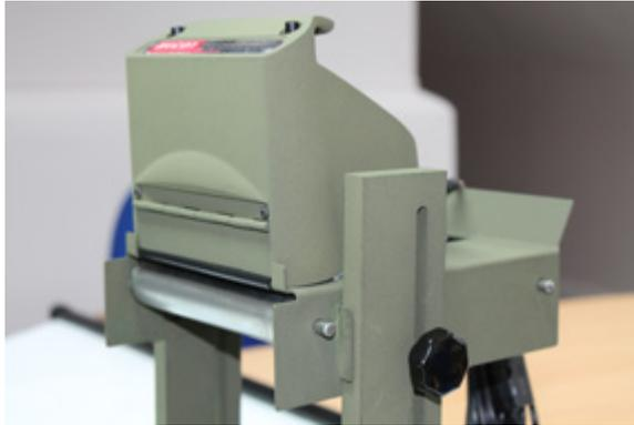
The height of the cradle is fully adjustable. To alter the height simply release the knurled screws, raise or lower the height of the cradle assembly and then re-tighten the screws.
